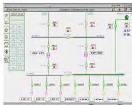
Fig. 14 Performance Test of Source 1 and 2 Failure Condition
