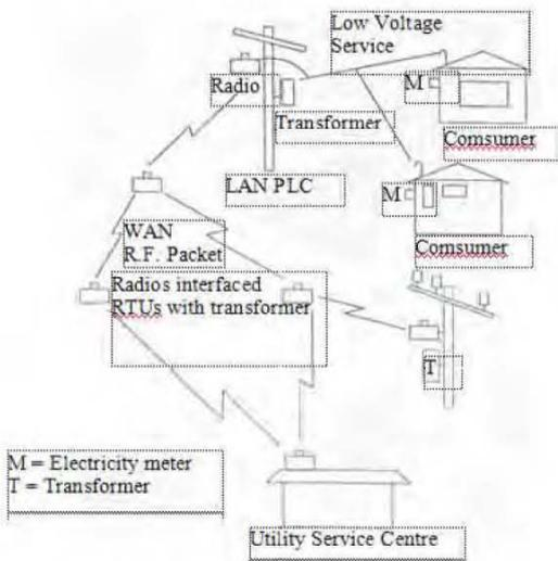
Fig. 4 Packet Switching Network (PSN)
